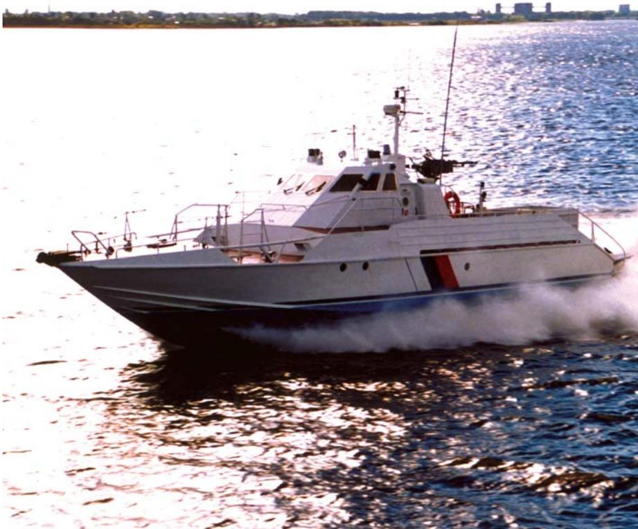
pitching and rolling motions and improve a sea-keeping ability at high seas. *Mirazh's* high characteristics were confirmed in the course of type ship trials in the Caspian Sea: in sea state 4 the ship accelerated to 40 knots with virtually no pitching and rolling.
